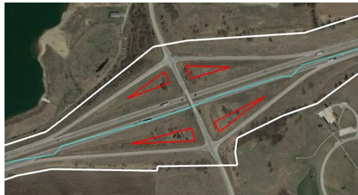
Figure 6. Example diamond interchange showing expected area for solar PV installation outlined in red
