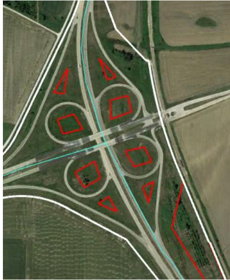
Figure 7. Example butterfly interchange showing expected area for solar PV installation outlined in red
