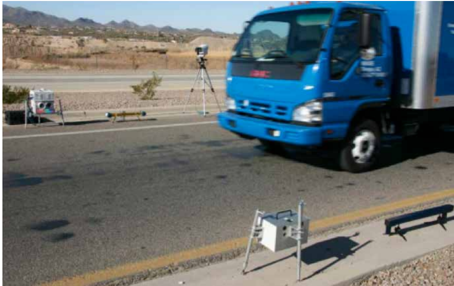
Figure 2: Enviro Technology Services AccuScan system [36]
