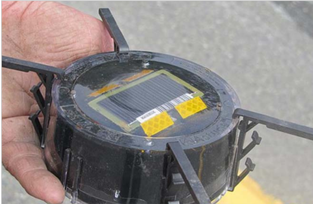
Figure 9 WSDOT solar reflector
