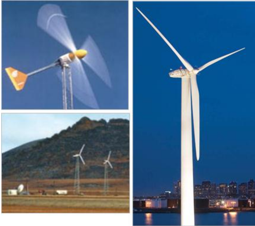
Figure 10 Examples of small-, mid-, and utility-scale wind turbines
